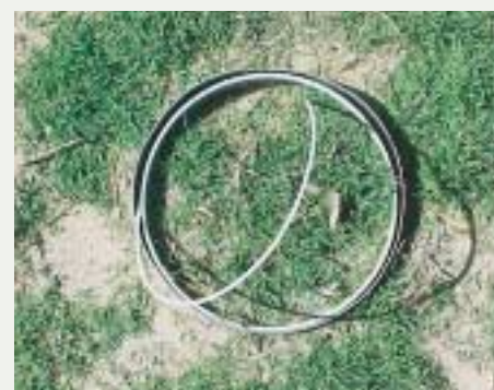
Installed lysimeter six weeks after planting
