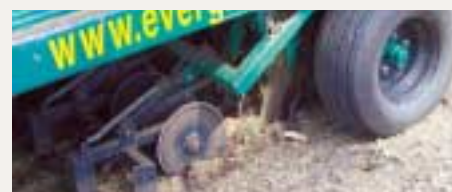
Burying the sprigs using a row planting machine
