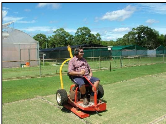
Plate 4: The Tru-Turf Greens Roller in operation on the 3.5mm cut and rolled plots
