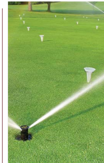
Catch cans are a quick, simple and cheap way of determining sprinkler uniformity
