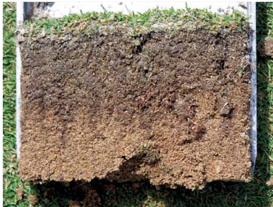
◀ Prior to start of the study, analysis of four randomly selected cores revealed a thatch/mat layer 0-2" deep with 5.8 per cent organic matter
