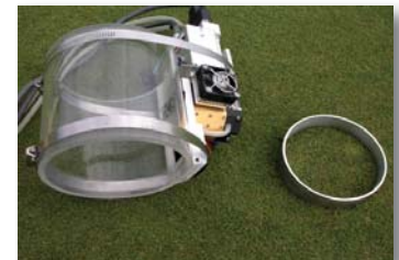
Photosynthesis and whole plant respiration were determined by enclosing the turf canopy in a transparent plexiglass chamber attached to a CO 2 analyser
