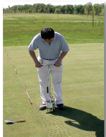
In the spring coring programme, plots were cored once annually using a hand aerifier containing seven 0.5-inch hollow tines which penetrated 3.5 inches
